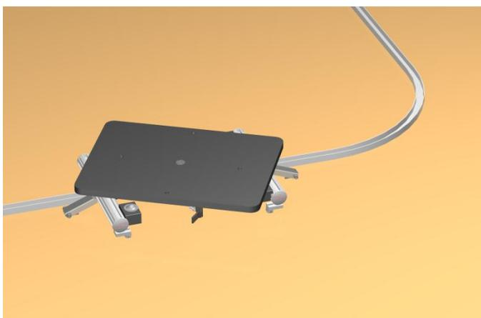
Finally you need to **position the pallet guides** and the pallet stoppers (pos. 8).
